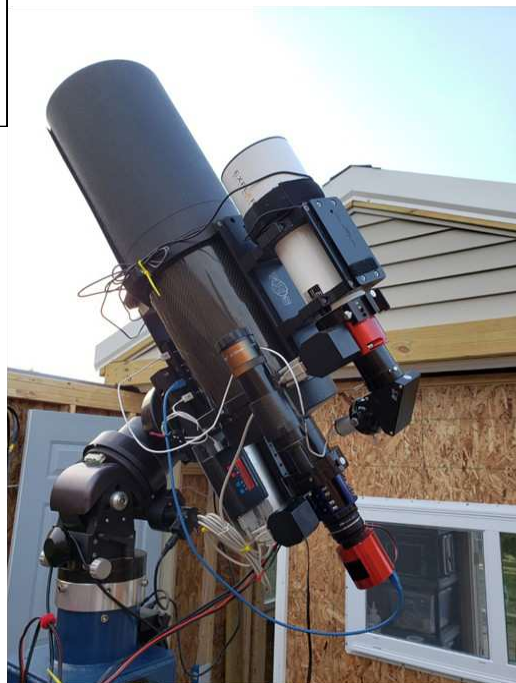
The pier riser was designed to fit on the existing pier anchor. The re-painted pier bolted to the top plate of the riser – easy peasy.
