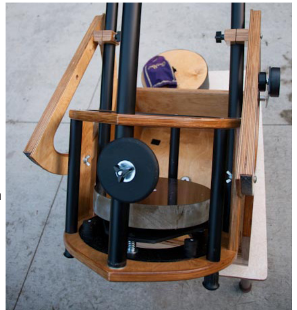
Close-up of the mirror box with the Kydex sleeve removed. Kydex replaces the usual wood walls of the box, lightning the scope dramatically.
