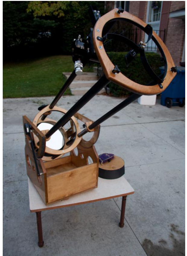
Minimal lumber makes a much lighter telescope. CNC cut parts makes for a tight and rigid fit. A Kydex oval opposite the focuser blocks stray light. Next page: Side view displays the open construction. Photos by the author
