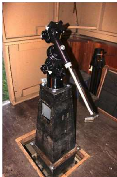
Next I had to order an adapter to mount the EQ head to my existing pier, which I bought through Telescope Support Systems (Clay Kessler and Jeff Thrush).
