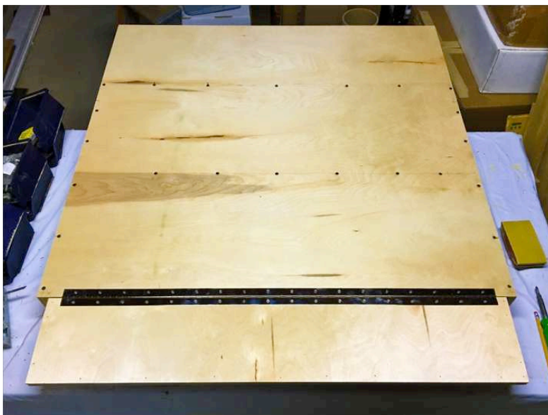
Make a frame out of some scrap plywood, and add a piece of ¼" plywood to the top. A flip-down panel, attached using a length of piano hinge, provides an even surface over which to roll the scope in and out, plus something to attach the ramps to. While loading/unloading it has to extend rearward past the front edge of the bumper, but flip up out of the way once everything is loaded so that the hatch can close.
