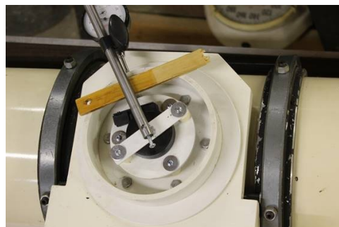
Centering the altitude encoder in the workshop.
