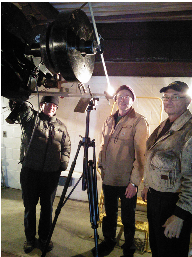
Two views of a mock-up mount for the Declination reaction arm. The left photo shows the structure in relation to the end of the Declination shaft. Pictured: (from the left) Don Fohey, Dave Jorgensen and Observatory Director Jack Brisbin. The right photo shows where the support for the Declination axis reaction arm will bolt to the telescope mount. The end of the Declination shaft is drilled and tapped. A bolt threaded into the hole and center drilled with a set screw will anchor the encoder shaft.
