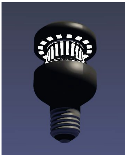
From below the mirrors reflect the light downward.
