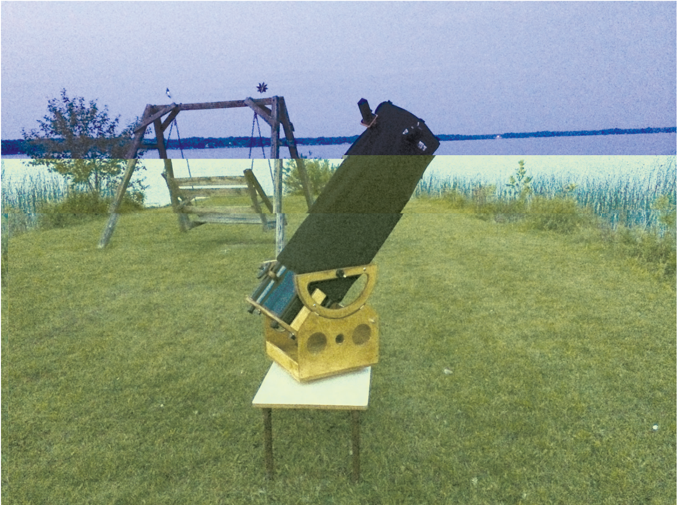
Paul's new scope, looking east in the evening twilight over Long Lake near Alpena, MI. The structure is an ultra-light kit from Dob-Stuff. The focuser is facing the camera. A Rigel 1x reflex finder is perched on the upper cage. Note coffee table. Photos by the author
