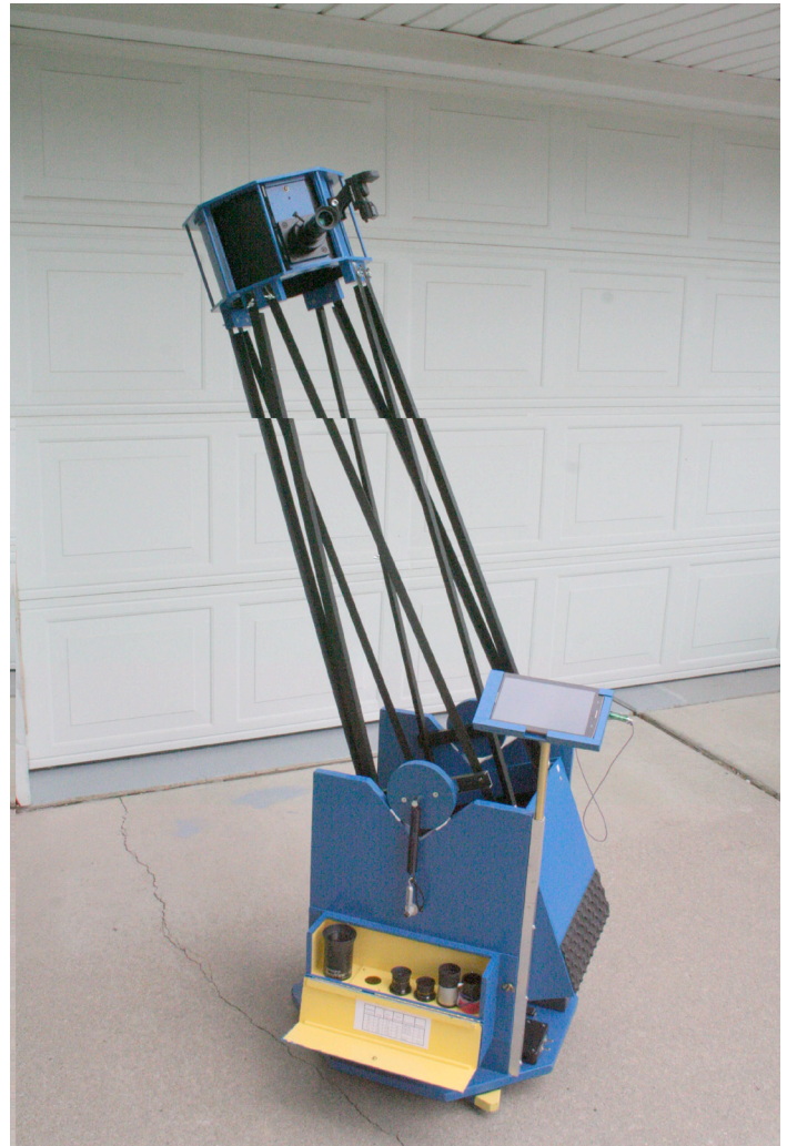
Above: Completed telescope. Note the eyepiece box and the stalk for Don's tablet.
