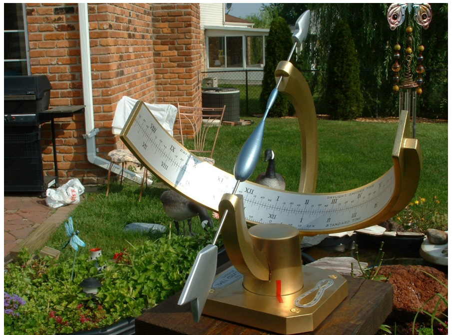
A sundial which features a linear dial and can be adjusted to show Standard Time. Built by the author. The gnomon in the shape of the analemma adjusts for the Equation of Time.
