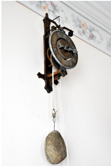
Thirteenth century crown clock reproduction with wooden gears. Note a rock is used as a weight, and the clock only has an hour hand. Not very accurate but better than a sundial. (One of my collection of clocks at home.)
