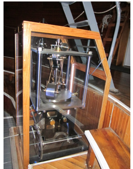
Clark Refractor Mechanical Tracking Apparatus
