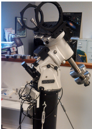
There is also the AP 1100 with a 110 lb. instrument capacity. The 1100 is a "portable" mount at 54 lbs. (less the pier) – so it could head out to Peach.
