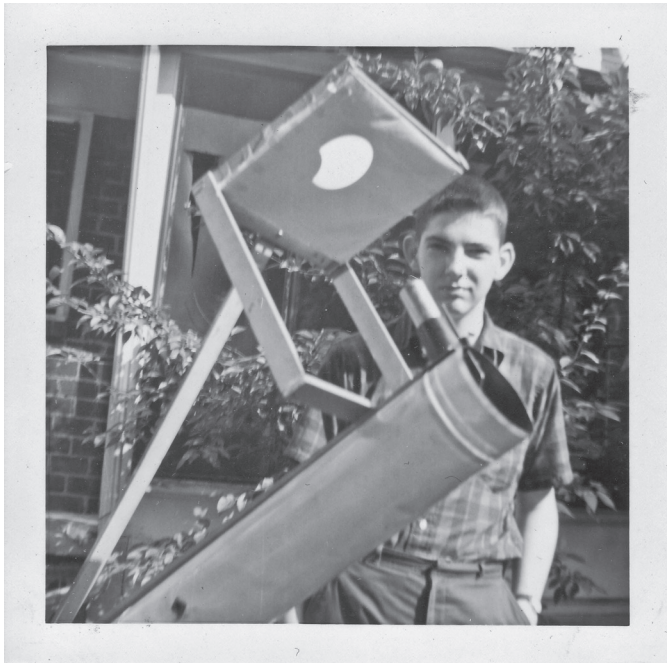
The optional solar projection screen was mounted for the partial eclipse of July 20, 1963. Photos provided by the author
