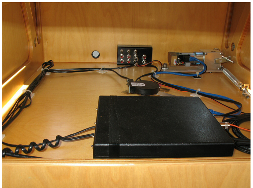
Here's the altitude drive side of the scope. The altitude drive motor is mounted to the left side of the rocker, and the altitude encoder is mounted to the center of rotation of the altitude bearing. The drive cable tensioning lever is mounted to the top of the newly added bearing extension as described in the text. The vertical gray bar holds the shaft of the encoder stationary while the scope moves up and down in altitude.
