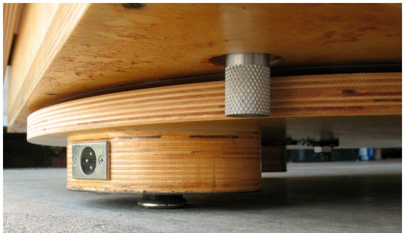
This picture shows the knurled roller (attached to the azimuth drive motor) protruding through the bottom of the rocker. Spring pressure pulls it against the edge of the round ground board. The roller needs a good "bite" into the edge of the ground board for the drive to work properly.
