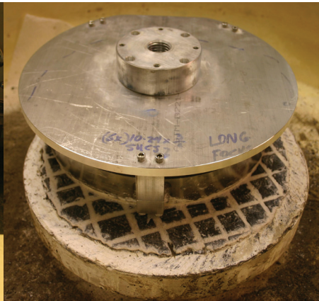
Mirror being polished out for the first time
