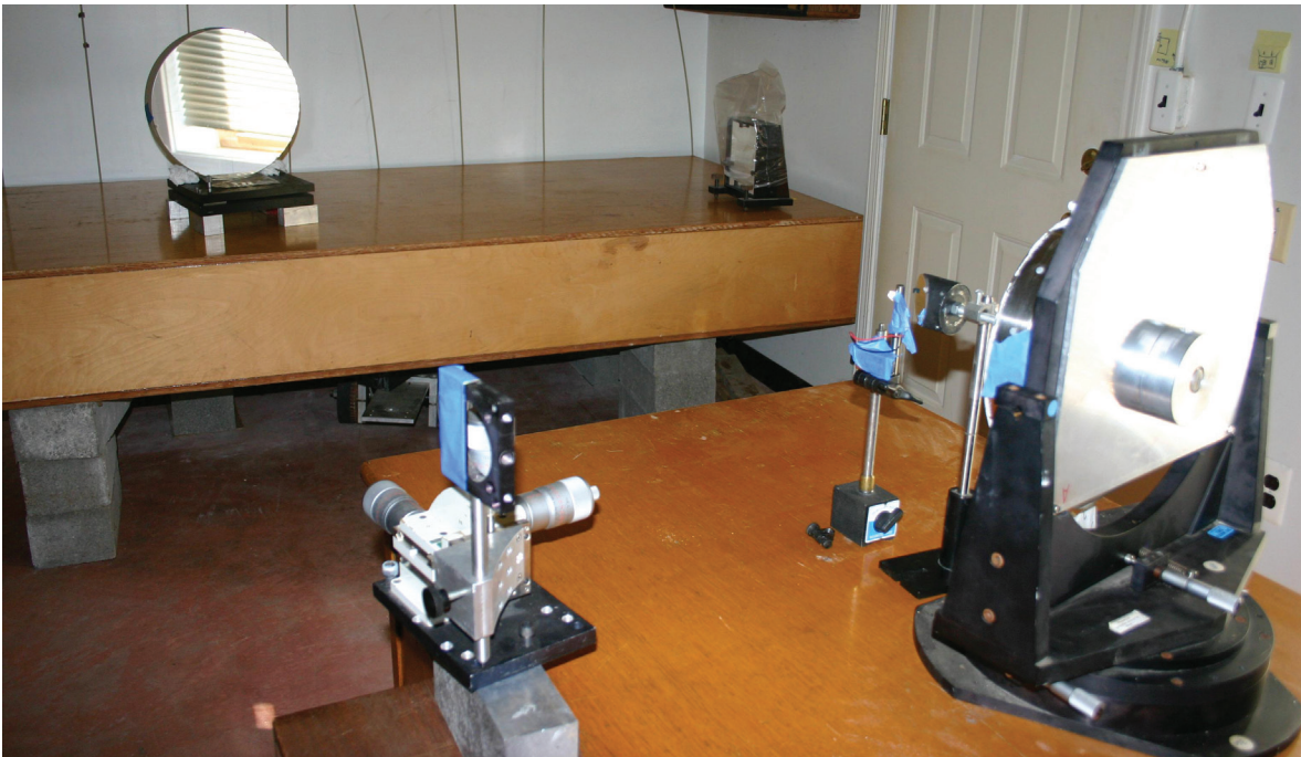
While the mirror was being polished, a mount was made to hold the mirror with its support plate on the optical bench.
