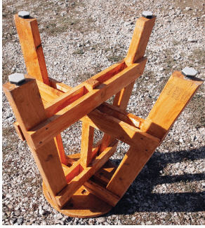
Underside of the barstool showing construction. Note adjustable feet.
