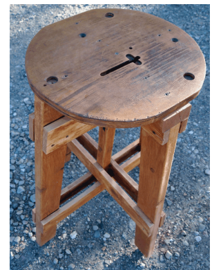
The top showing 3 cups for the Starblast feet. Cups could be added for additional scopes. The extra holes are from a previous use of the plywood.
