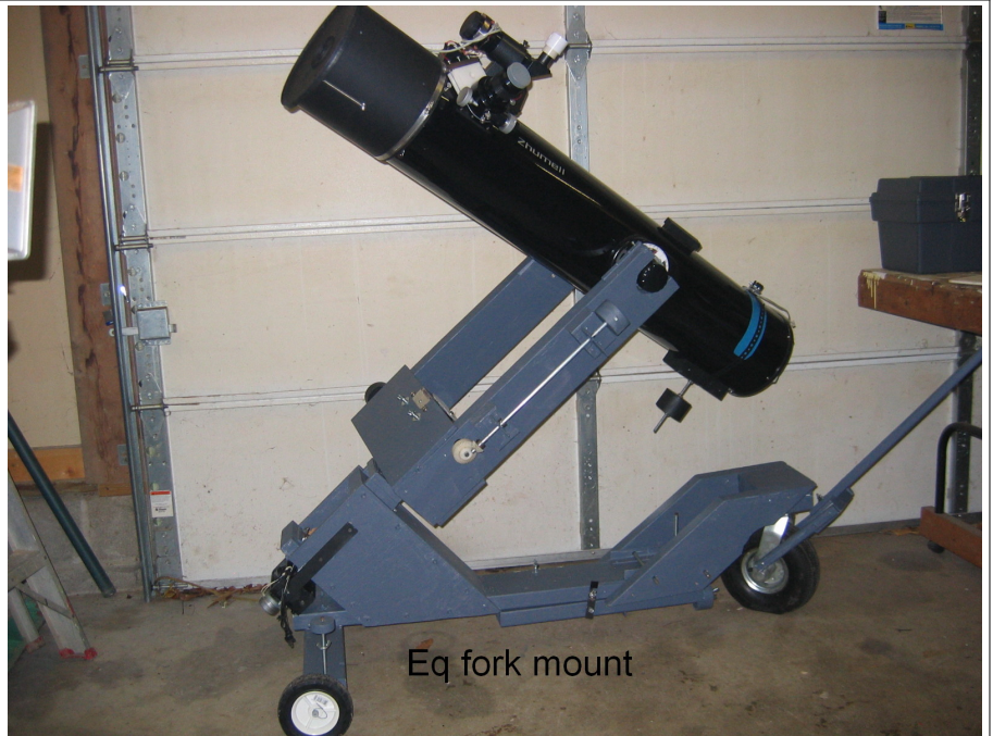
David Jorgensen's homebuilt fork mount, for his 8" f/6 Newtonian . Read the article on pages 6 and 7.
