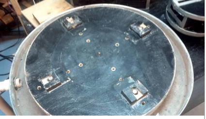
Wa La, the mirror is always in the center of the turntable and in the same spot. Before placing the mirror on the table, I put down a cushion for a soft support for the mirror *(see picture below)* and adjust the height of the acorn nut just enough so the mirror hole can find it but not resting on it. The cushion is cut from a cheap thin yoga mat.
