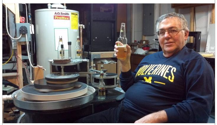
Polishing is quite easy because I don't have to sit there. I made a cerium dispensing system consisting of a tank, a peristaltic pump and an on-off timed relay. Polishing out a 12" blank takes three to five hours, after which initial testing can be done. I use the Ronche test at this point.
