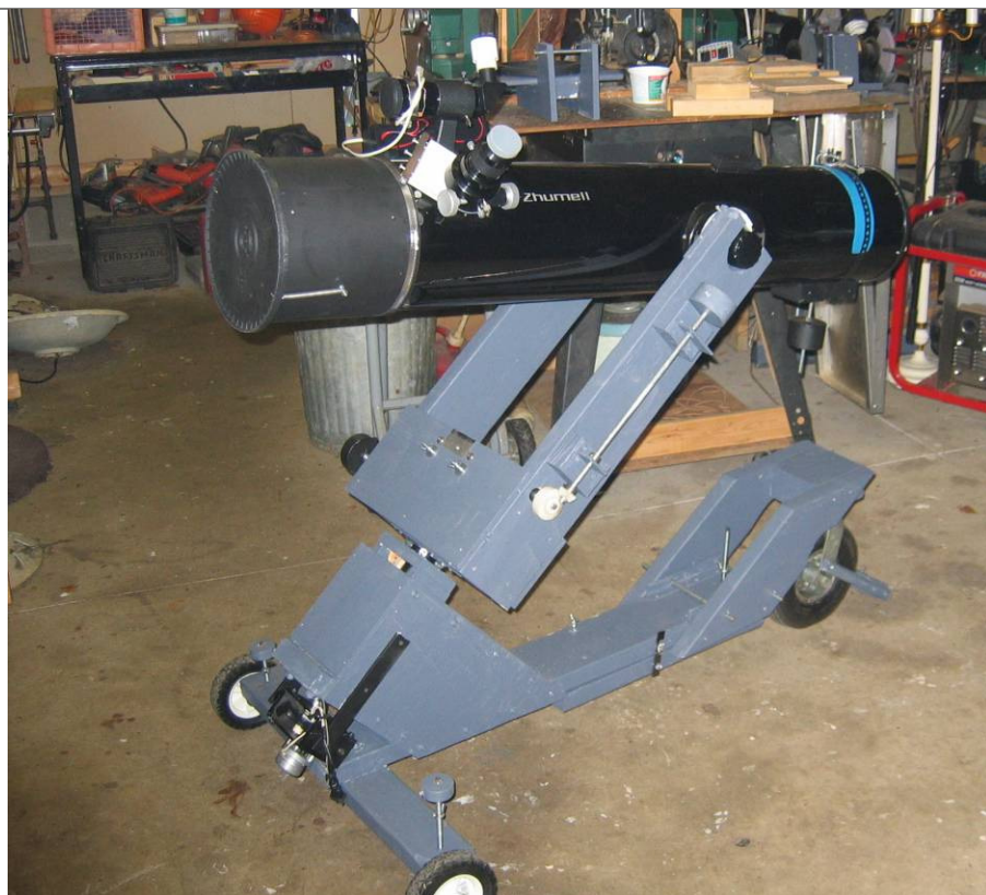
David Jorgensen has made an EQ yoke mount for an 8" f/6 Newtonian, and promises an article soon.
