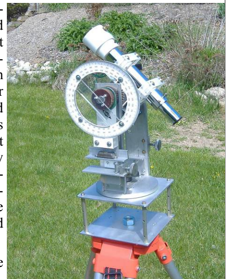
Figure 1 Zenith Angle Measuring Theodolite
