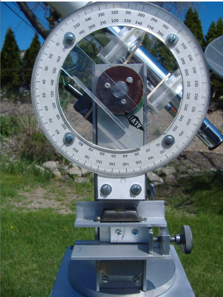
Figure 2 Close-Up Showing Vernier Dial and Spirit Level
