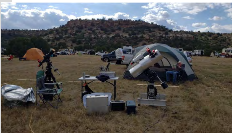
Roger Tanner brought his 10" f/3.9 astrograph on an iOptron CEM70g, and I had my 4" refractor on my Losmandy G11. We were both doing imaging all week.
