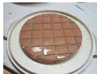
8 inch synthetic pitch tool with polish.
