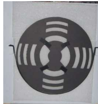
Zone Mask. I would measure zones 1, 3, 5, 7 and then rotate for zones 2, 4, and 6
