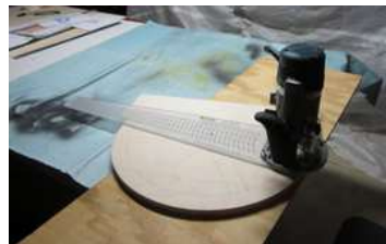
Cutting out altitude rocker
