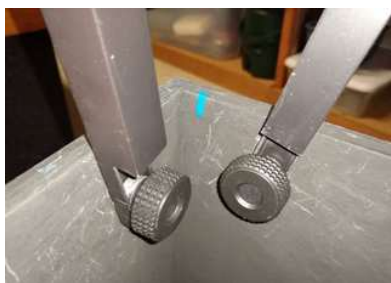
Truss Pole Attachment to Mirror Box
