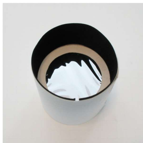
Completed filter. It's a snug fit over the end of the lens. Black flocking will help prevent stray reflections.
