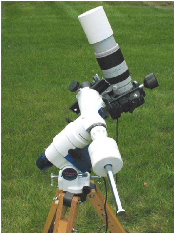
My eclipse photography setup. A Canon 7D crop-sensor DSLR, 100-400mm zoom lens, fitted with a solar filter. The camera is mounted on a Vixen Great Polaris 2 GEM with RA drive using a heavy-duty Manfrotto 486 ball mount.
