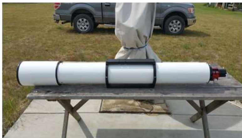
Then I added the baffles, tailpiece/focuser, rings and dew shield. It went very quickly.
