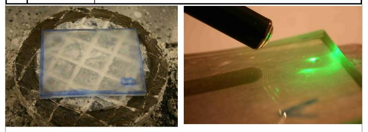
out completely and evenly. In the picture with the laser pointer, the beam passes through the polished surface with very little scatter before hitting the ground surface on the back of the mirror. You have to look very closely to see the scatter off the front surface, and lasers are very bright.
