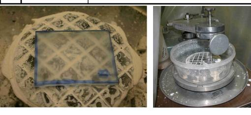
Because these mirrors were part of a prototype which needed to be made fast, rather than good, as long as good was good enough to prove the concept, they were ground fast polished and fast. Their edges polished out first, but a dimesized spot in the middle never did polish
