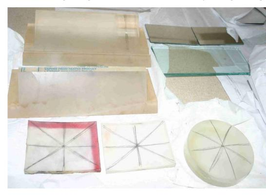
Until recently, I had only tried the first method. However, running a finished element through a diamond saw, and then grinding the edges until they are square and to size, requires an excellent surface protection tape and a great deal of luck to prevent scratches. I knew the success rate of that approach, and I decided to try the second method.
