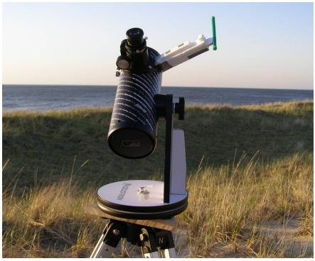
The primary mirror seems to be glued to the bottom of the tube and not adjustable. The secondary is attached with a single vane and can be collimated.
