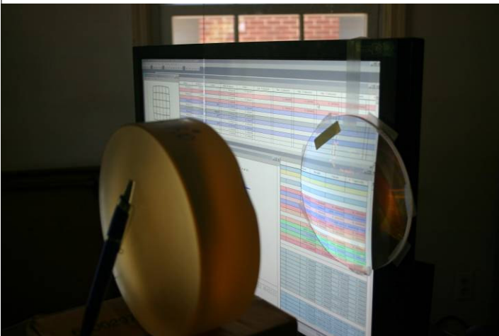
Figure 3. Mirror, large lens, and beamsplitter cut from window glass. Figure 4. Mirror, 45 degree beamsplitter, lens and display.
