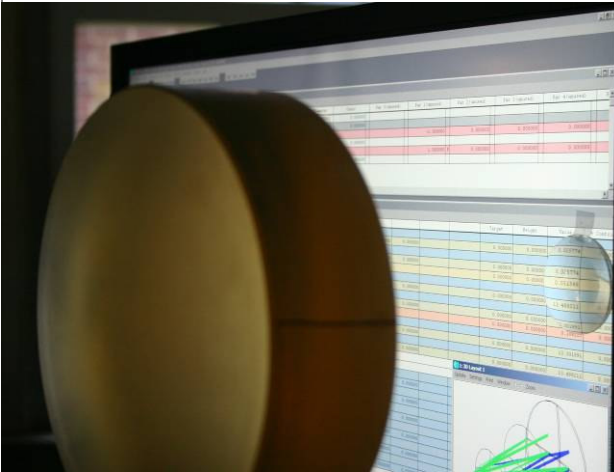
Figure 1. 6" f/1.4 mirror and field flattening lens
