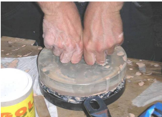
The pitch lap was formed using a mirror on top technique. The pink solution is cerium oxide.
