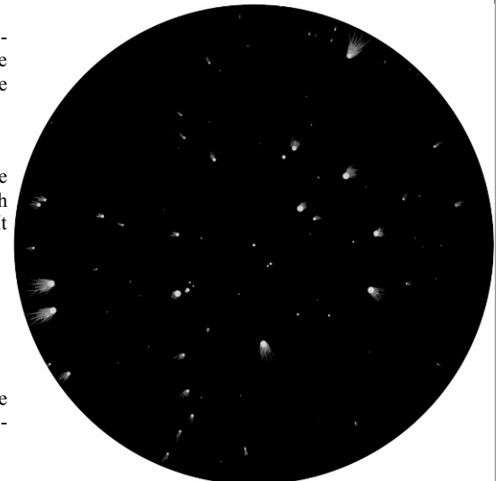
Fig. 1 - Coma in a Newtonain reflector
