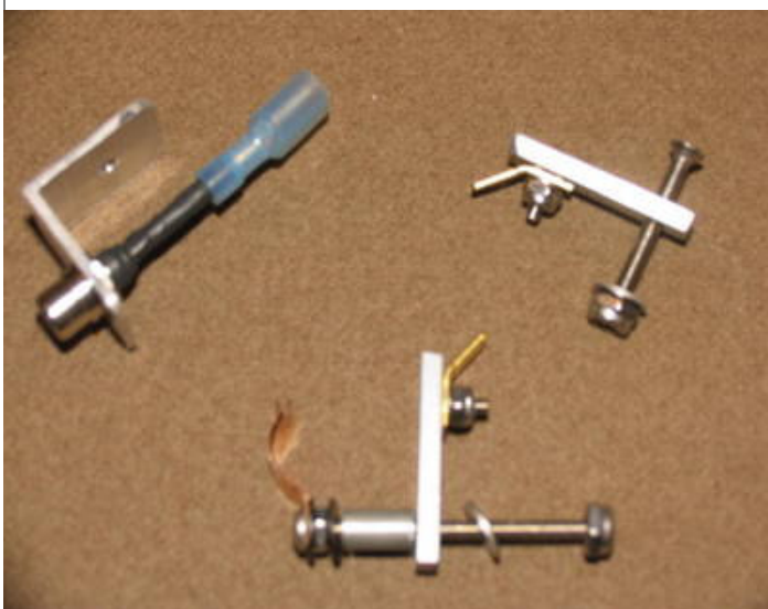
Figure 11: Powered Truss System Terminals
