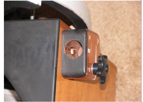
Electrical Tab in Truss Block
