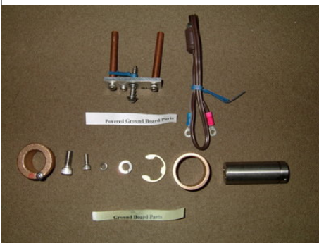
Ground Board Electrical Hardware
