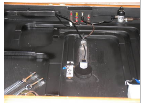
Rocker Box Showing Power Panel
