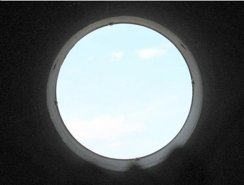
Fig. 4 Looking up through the tube at the open sky, showing the difference between flocking and flat black paint. The bright ring is where it is painted with the flattest flat black paint commonly available, the rest is flocking. (The painted portion is behind the primary mirror where it doesn't matter.)
