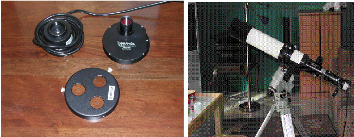
Clockwise from upper left: Camera with nosepiece removed, Filter Wheel, Kendrick "KwikFocus"
