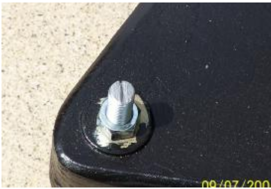
Figure 3 Polar alignment and or leveling screws.
