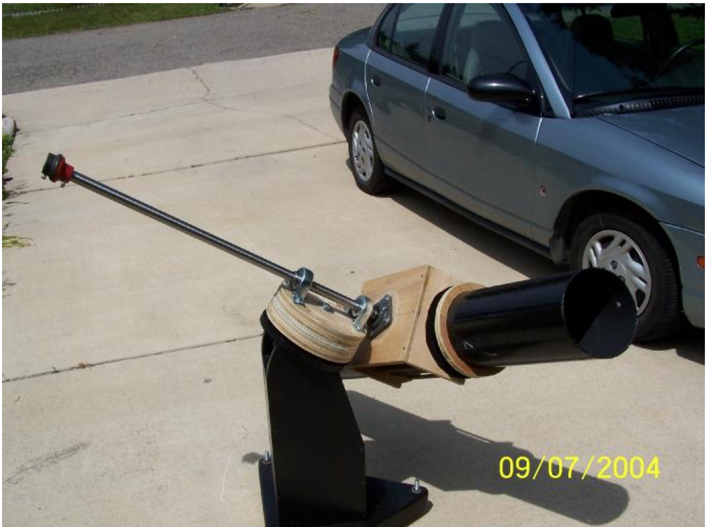
Figure 1 Cradle, declination axis pillow blocks on old polar head
