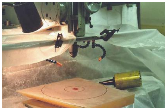
Glue the glass to the aluminum plate.
