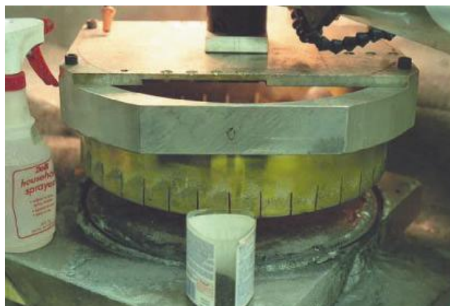
Cut the outside diameter.
