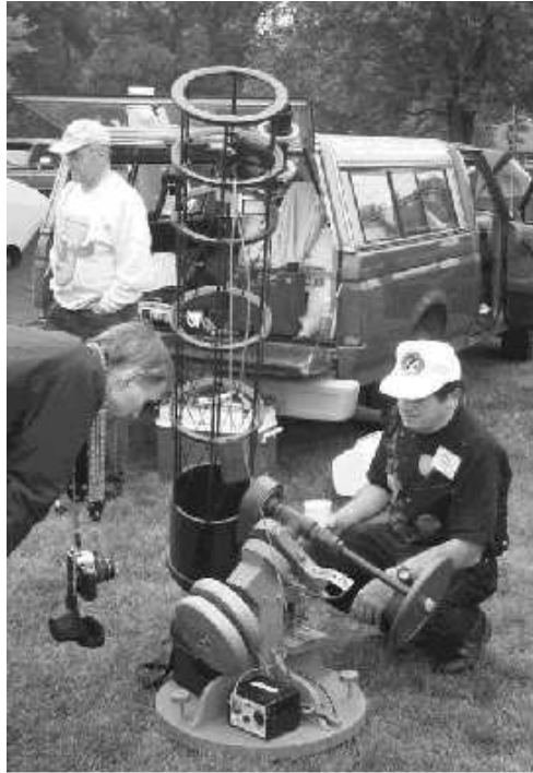
Very interesting scope. Tube is tension wires (motorcycle spokes) threaded through cast rings.
