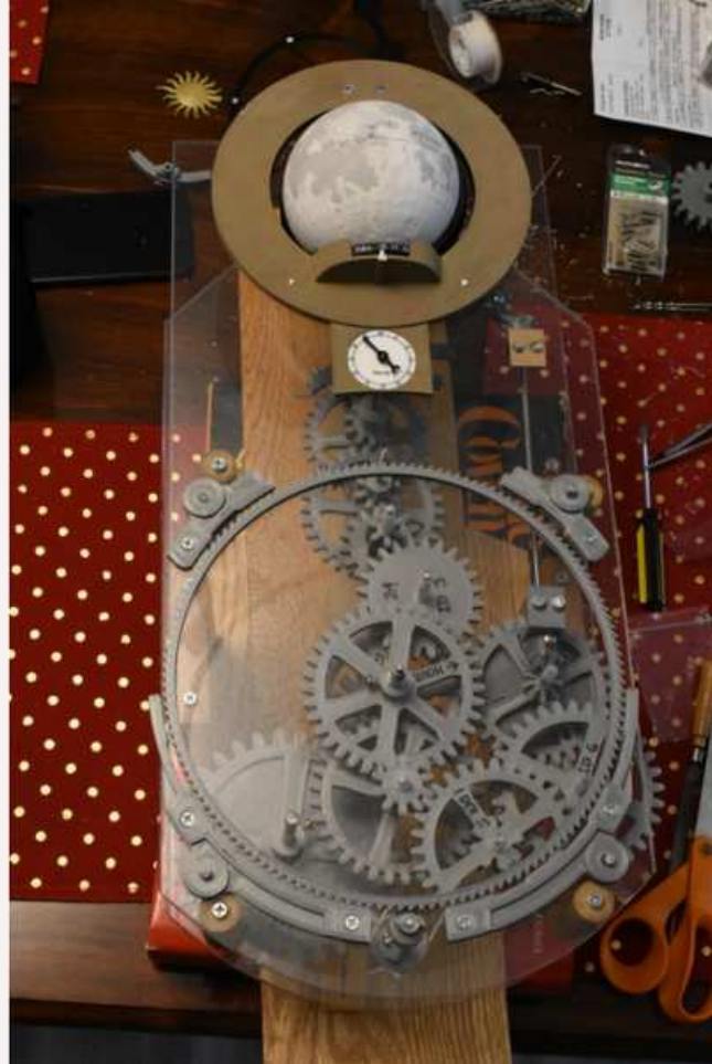
ABOVE: Clock gear assembly. The saw tooth ring gear is held in place with curved guide plates. At the bottom of the ring gear is 2-bladed paw gear which rotates every 5 days advancing the star chart 2 times. The Moon globe is stationary showing the same face to the viewer with a separate cover to display the moon phases.
