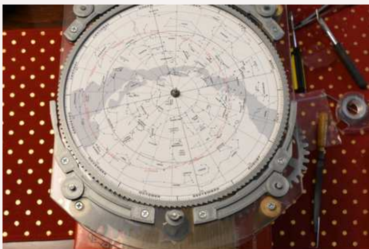
ABOVE: This photo shows the star chart attached to the ring gear. Chart was drawn using Corel Draw.
