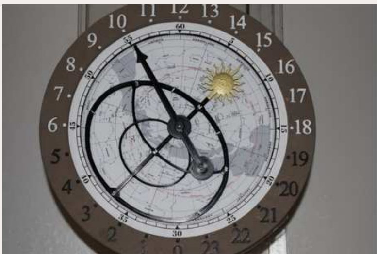
ABOVE: Detail view of star chart dial. The red circle is the ecliptic with dates of where the sun is each year. Of course, this varies slightly from year to year, but it gives a good indication of sun rise and sun set times.
