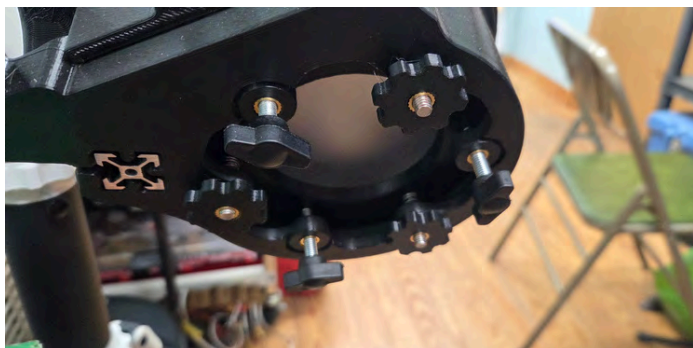
ABOVE: COLLIMATION KNOB LEFT: PRIMARY COLLIMATION SCREWS,
